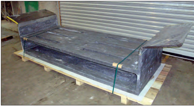
Fig. 9: Compact anode ready for transport at JL Goslar GmbH
